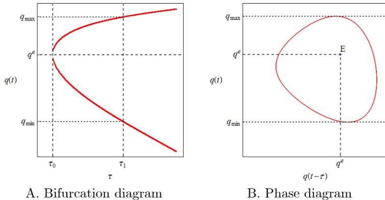
Figure 3. Emergence of a limit cycle
